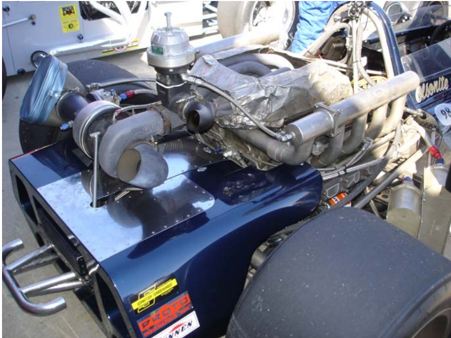
Indy 4 cam Turbo Ford powering #42
